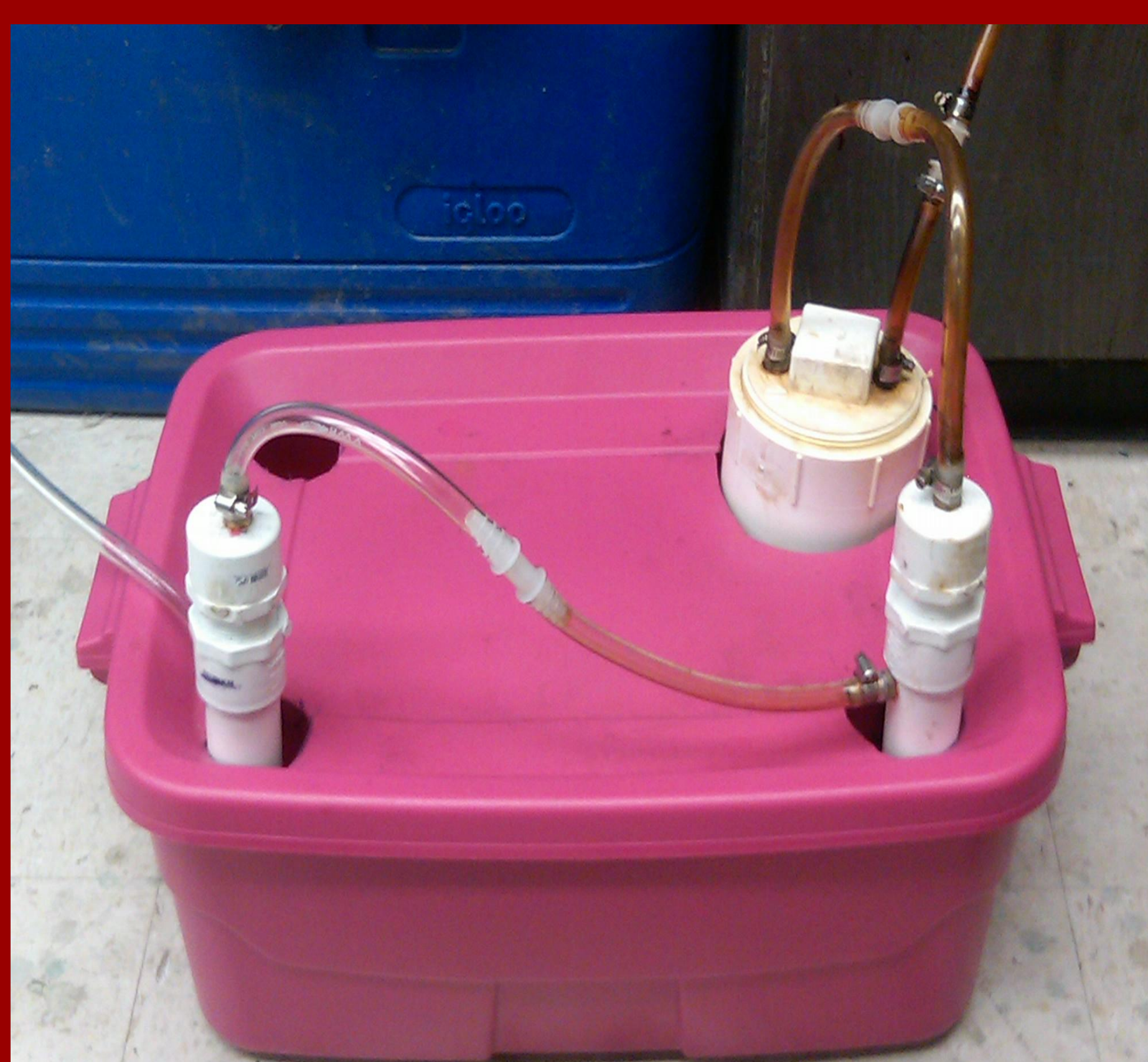
Figure 3. Bio-oil collection and acid trap setup.
