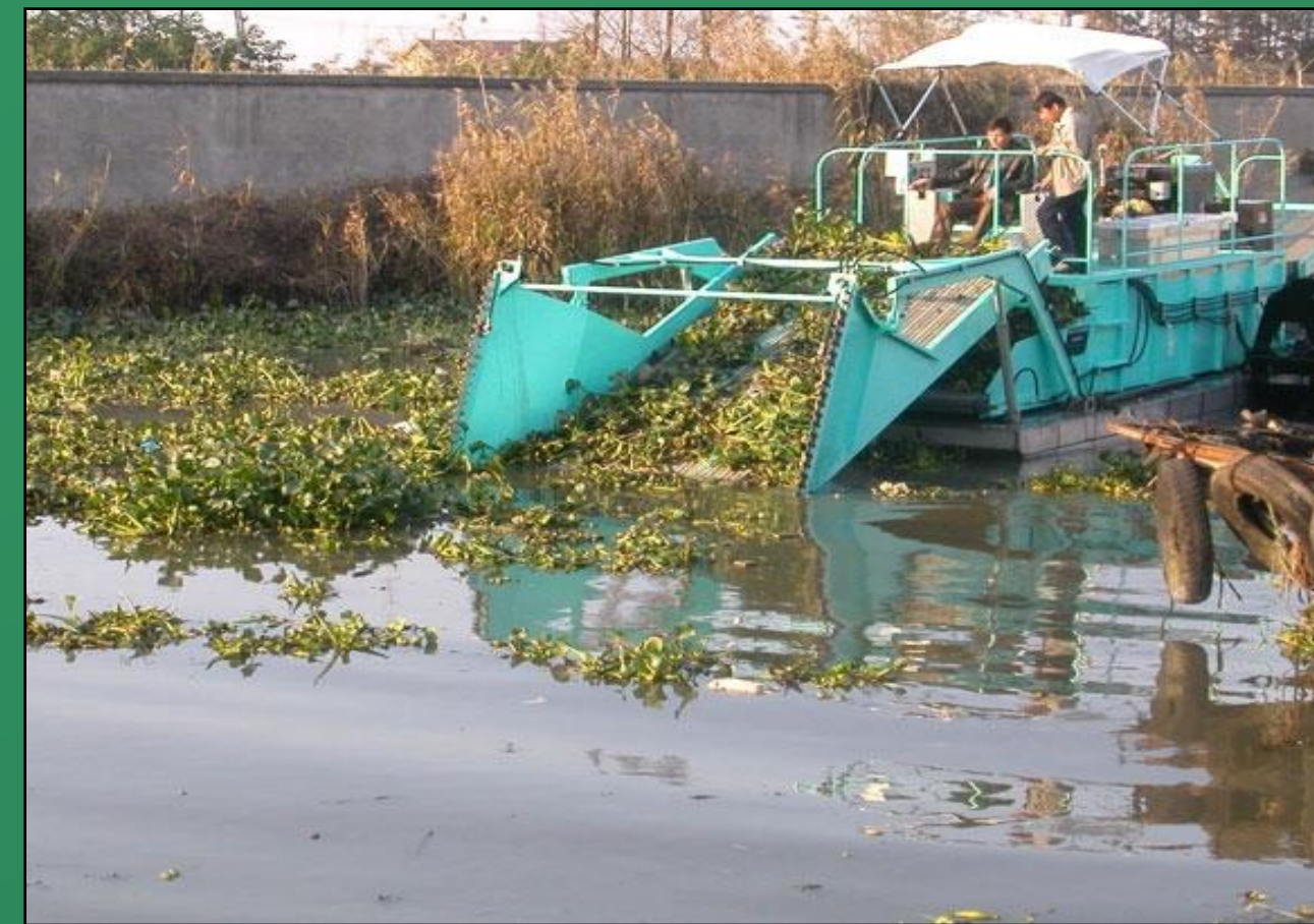
Figure 1. Typical weed harvester as used on Pewaukee Lake. http://aquaticweedharvester.com/photos.htm
