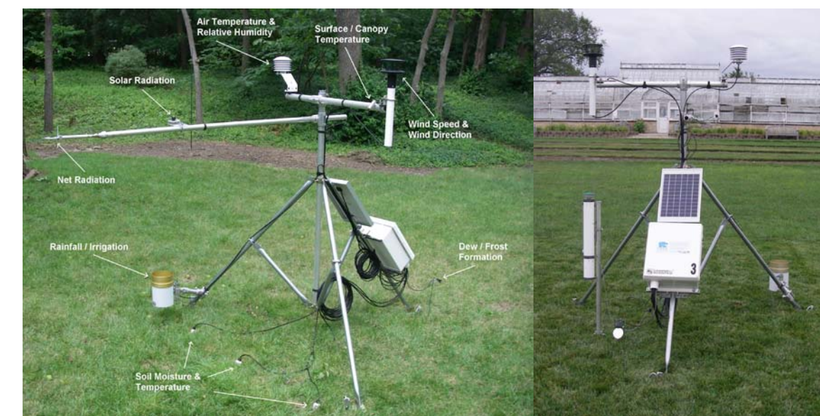
Fig. 1. Left: A tripod deployed in a lawn with instrumentation labeled. Right: Taking measurements in the Kansas State University Gardens.
