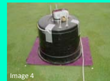
Image 4. Light box mounted to frame with golf tees marking corners
