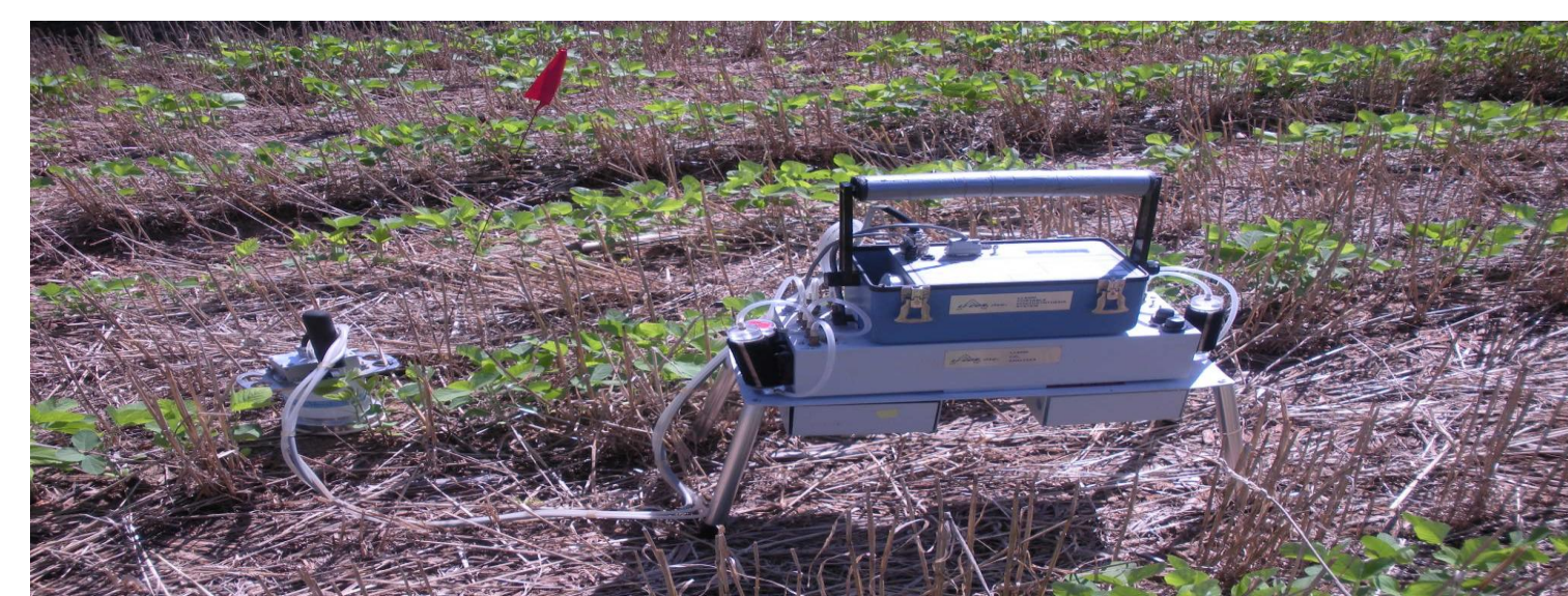
Fig. 2. CO 2 measurement using LI-COR 6200
