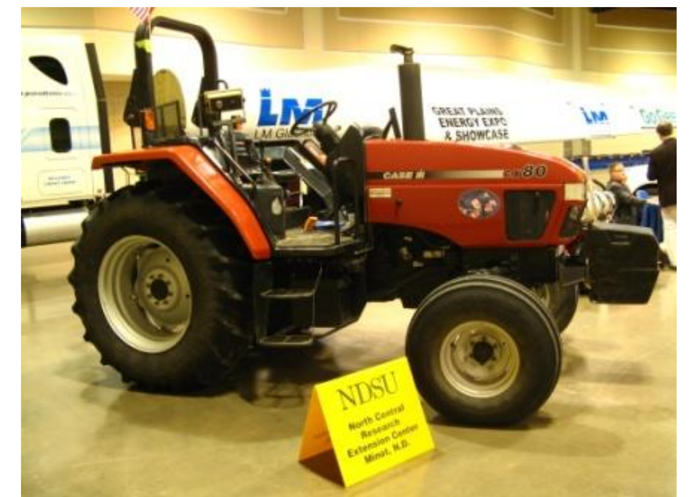
Case IH diesel tractor after 6 years Operating on 100% bio-diesel
