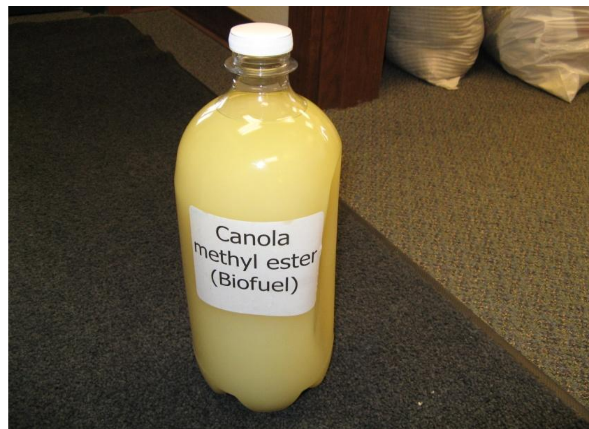
Canola methyl ester after 12 hours at 5 degrees Fahrenheit
