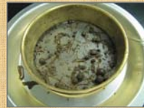
Figure 6. Wet sieved root biomass after dispersion by 10 % HMP.
