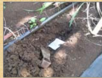
Figure 15. Litterbags will be buried at 10 cm depth in 45° angle.
