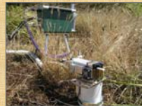
Figure 5. Li 6400 portable photosynthesis system with soil respiration chamber.
