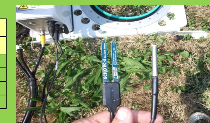
Figure 8: ECH2O Soil Moisture Probe (left) Omega Soil Temperature Probe (right)
