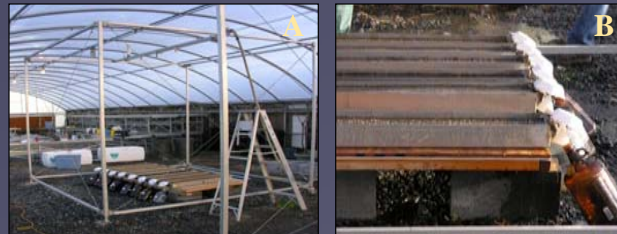
Figure 1: Rainfall simulation apparatus (A); and Collection of runoff water during rainfall (B)
