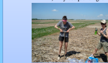
Figure 2: Four subsamples across a diagonal transect were collected using a 5cm diameter soil corer.
