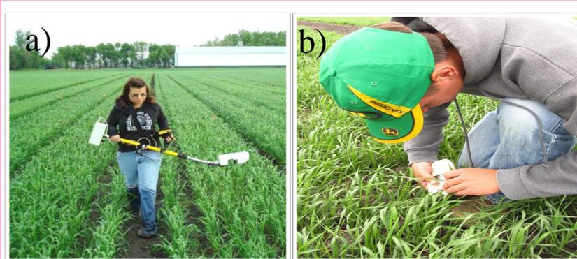
**Figure 1:** Diagnostic tools used for predicting protein content: a) Greenseeker Model 505; b) CCM-200 Chlorophyll meter. Measurements taken at the Zadoks GS 16.
