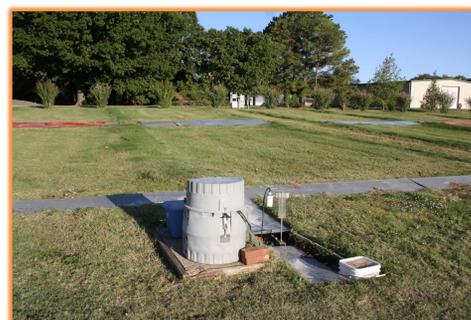
Photo 2. Automatic Sampler and Ultrasonic Sensor
