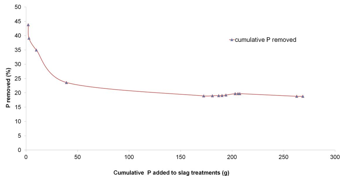
Figure 2. Proportion of cumulative phosphorus (P) [(cumulative P in runoff that entered the slag filters – cumulative P that exited the slag filters) / cumulative P that entered x 100] removed from 14 natural and simulated rainfall runoff events from 11 Mar through 30 Sep 2012.
