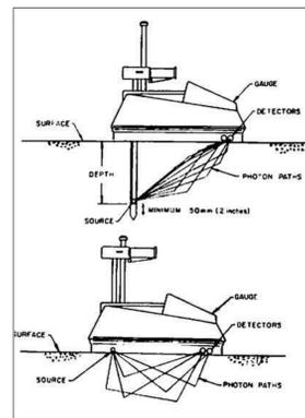
Figure 2. Direct transmission (top) and backscatter geometries (bottom) for nuclear density gauge. (Troxler Electronic Laboratories, Inc.)
