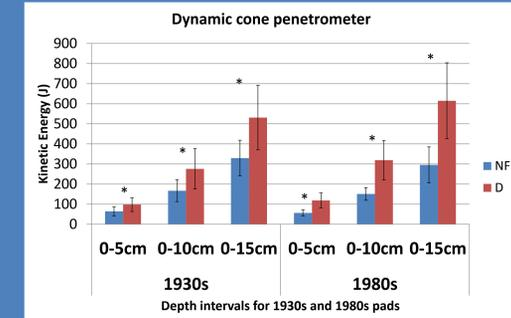
Figures 5a-5d. DSP data for conventional gas sites (\* indicates significance at alpha=0.05; NF= native forest; D=disturbed) a.) Bulk density from core method b.) pocket pentrometer c.) dynamic cone penetrometer d.) dry density from Troxler gauge
