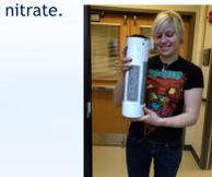
Figure 4: Constructed Wetland Soil Column: 4 inch PVC pipe with drainage holes and mesh covering.
