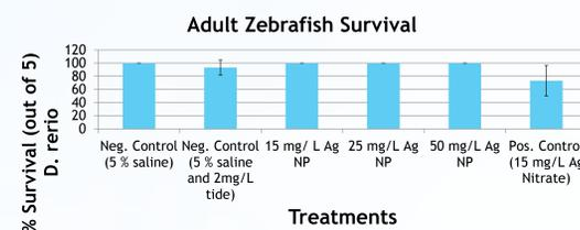
Figure 1: Adult zebrafish survival expressed as a % after a 7 day exposure. Each bar is the average of three trials of 5 fish (2 male, 3 female) per lab-scale constructed wetland bucket. Error bars indicate standard deviation; Kruskal-Wallis test gave a p-value of 0.134 between treatments.
