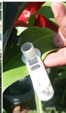
Fig 2. Dark adapted measurement of Fv/Fm
