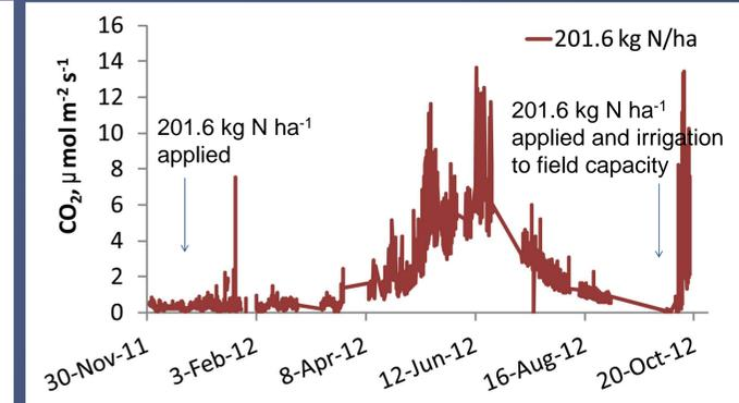
Measurements were conducted 24/7/365. The flush of N<sub>2</sub>O was observed in the spring, and also in the fall immediately following the irrigation and N fertilization experiment. CO<sub>2</sub> peaked out during May-June period prior to drought, and immediately after initial wetting.
