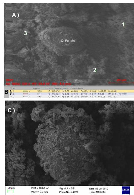
Figure 2. A) MEV-EDS image SE and B) microanalyses of Fe-Mn nodules in the clay fraction of the P37A soil. C) Nodular habit Fe-Mn oxides in the sample. (Photos by Olívia Graziela Gelioli do Carmo)
