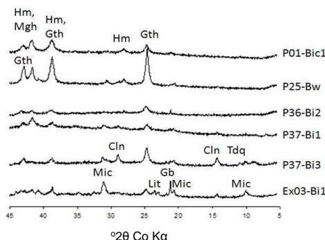
Figure 1. XRD patterns - oriented clay of soils from ferruginous dolomite of the Gandarela formation (Hm: hematite, Mgh: maghemite, Gth: goethite, Cln: kaolinite, Tdq: todorokite, Mic: mica, Lit: lithiophorite, Gb: gibbsite)
