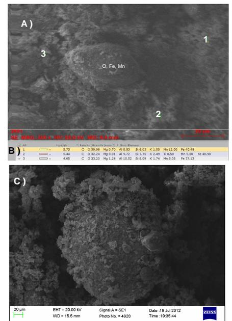
Figure 2. A) MEV-EDS image SE and B) microanalysis of Fe-Mn nodules in the clay fraction of the P37A soil. C) Nodular habit Fe-Mn oxides in the sample. (Photos by Olívia Graziela Gelioli do Carmo)
