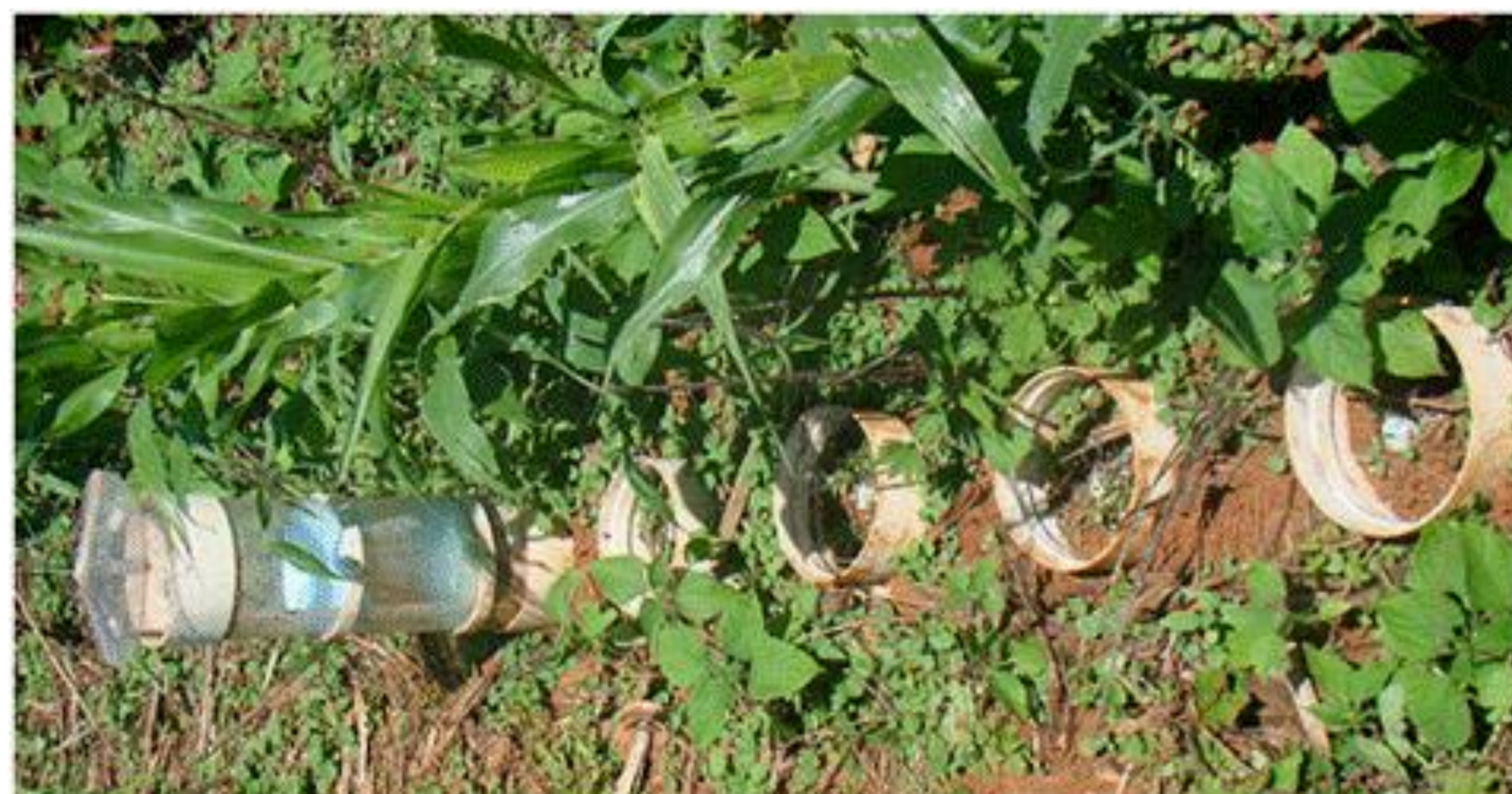
Figure 1. Evaluation of ammonia volatilization from fertilizers through semi-open collector in dynamic form.
