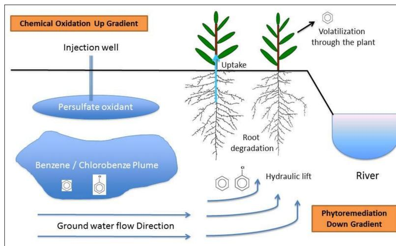
Fig. 1. The remediation plan to use Persulfate Oxidation and Phytoremediation to clean up benzene compounds in a former pesticide plant in Southern Brazil.
