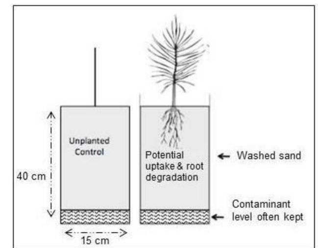
Figure 6. Pots in the greenhouse experiment with plant and unplanted control. Washed sand is used to reduce sorption.
