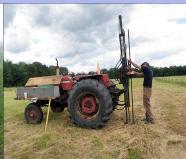
Fig. 3- Giddings hydraulic soil sampler used to extract soil cores.
