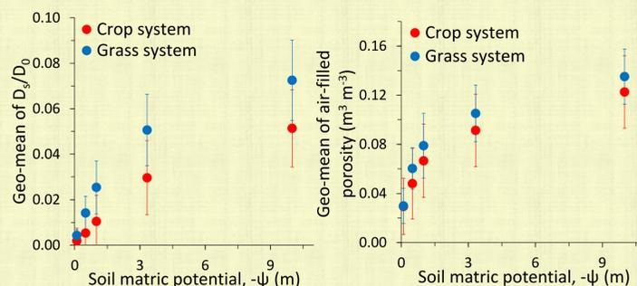
Fig. 2: Geometric means of relative gas diffusivity and air-filled porosity in crop and grass systems at different soil matric potentials. Bars indicate standard deviation.
