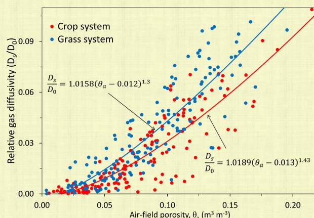
Fig. 3: Relative gas diffusivity as a function of air-filled porosity  $\theta_a$  in crop and grass systems measured at five soil water matric potentials: -0.1, -0.5, -1.0, -3.3, and -10 m.
