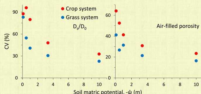
Fig. 4: Spatial coefficient of variation (CV) of relative gas diffusivity and air-filled porosity in crop and grass systems at different soil matric potentials.
