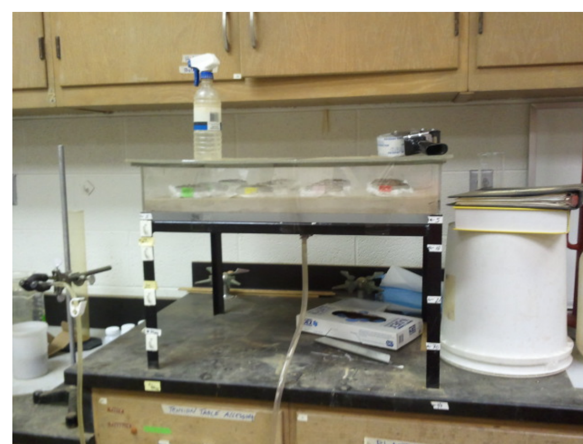
Figure 3. Constructed tension table to apply suction to achieve desired gravimetric potentials.
