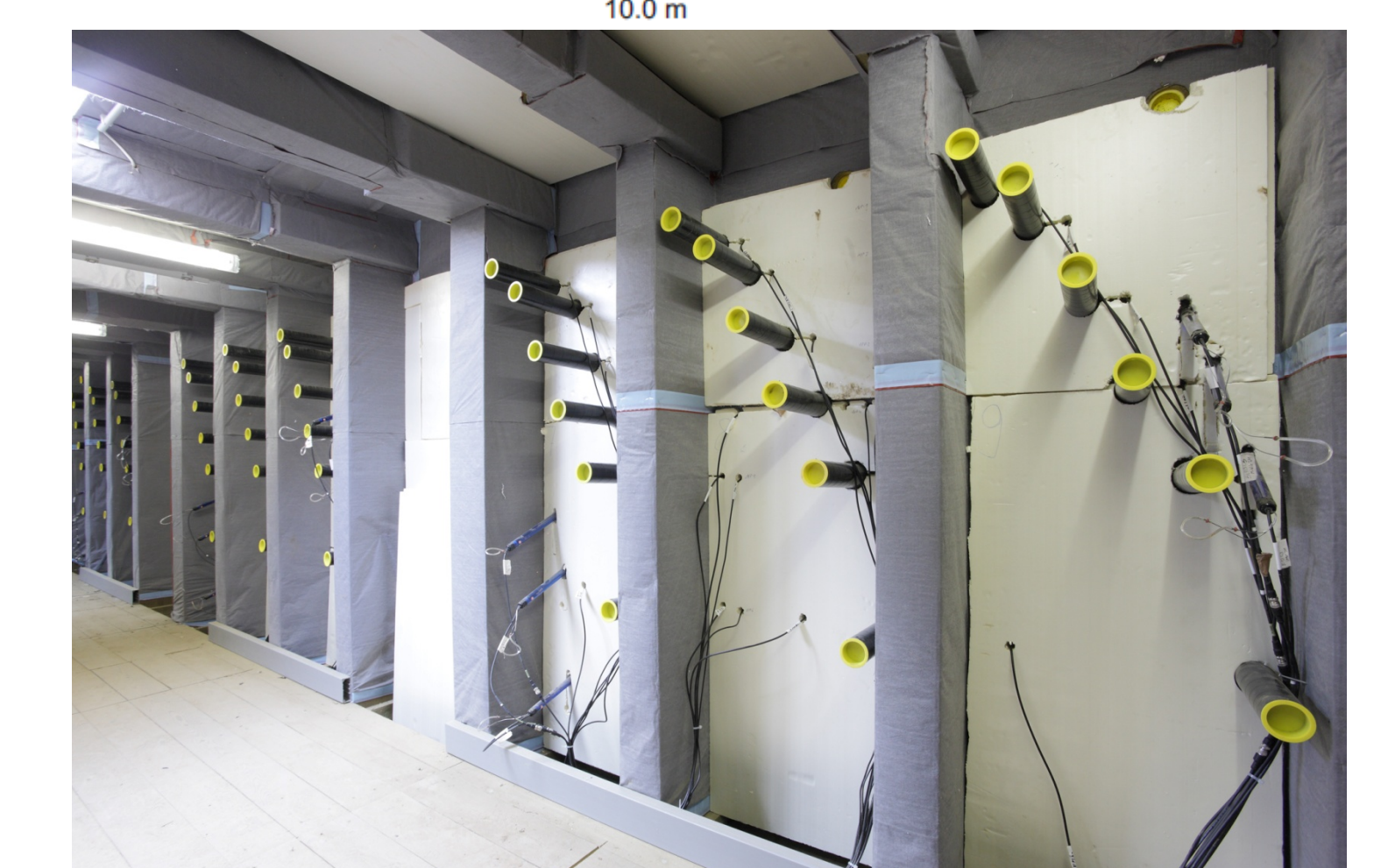
Schematic sketch (top) and photo (bottom) of the TDR trench used for field experiments. Field shows high electromagnetic noise due to ground currents.
