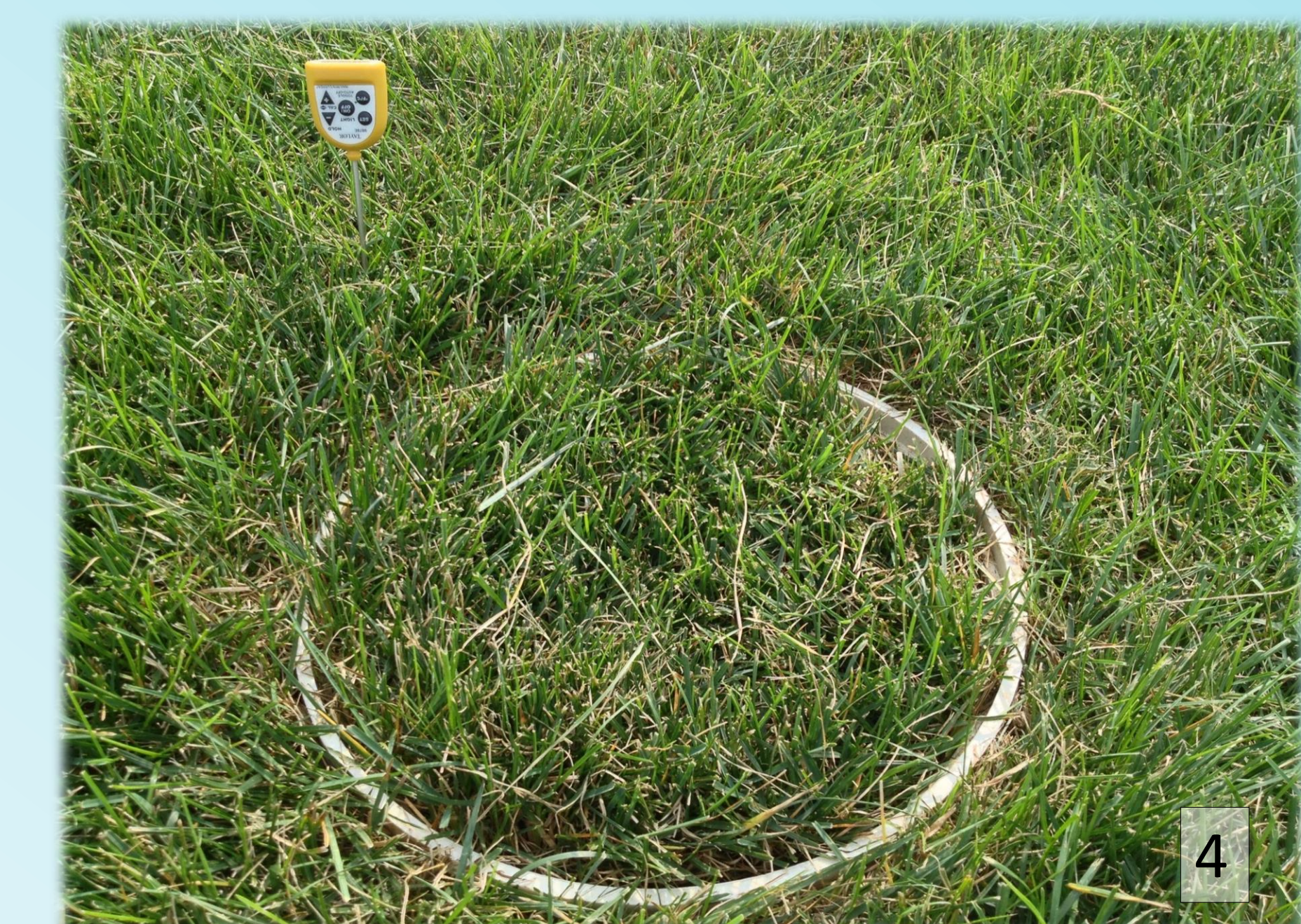
Figure 3. Picture showing the field sampling instruments: INNOVA photoacoustic gas analyzer and flux chamber. Figure 4. Trace gas collars were installed permanently in field, ~2cm above ground and 13cm below ground.
