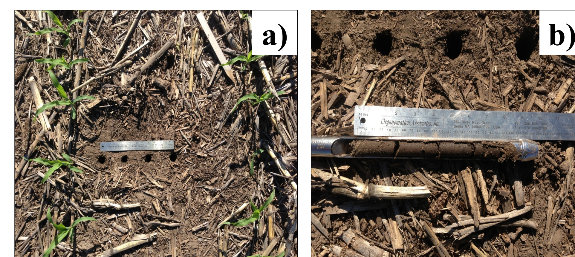
Fig 4. Soil sampling scheme with locations (a) and depths (b). Samples were analyzed for inorganic N (NH 4 + and NO 3 - ), data not shown.
