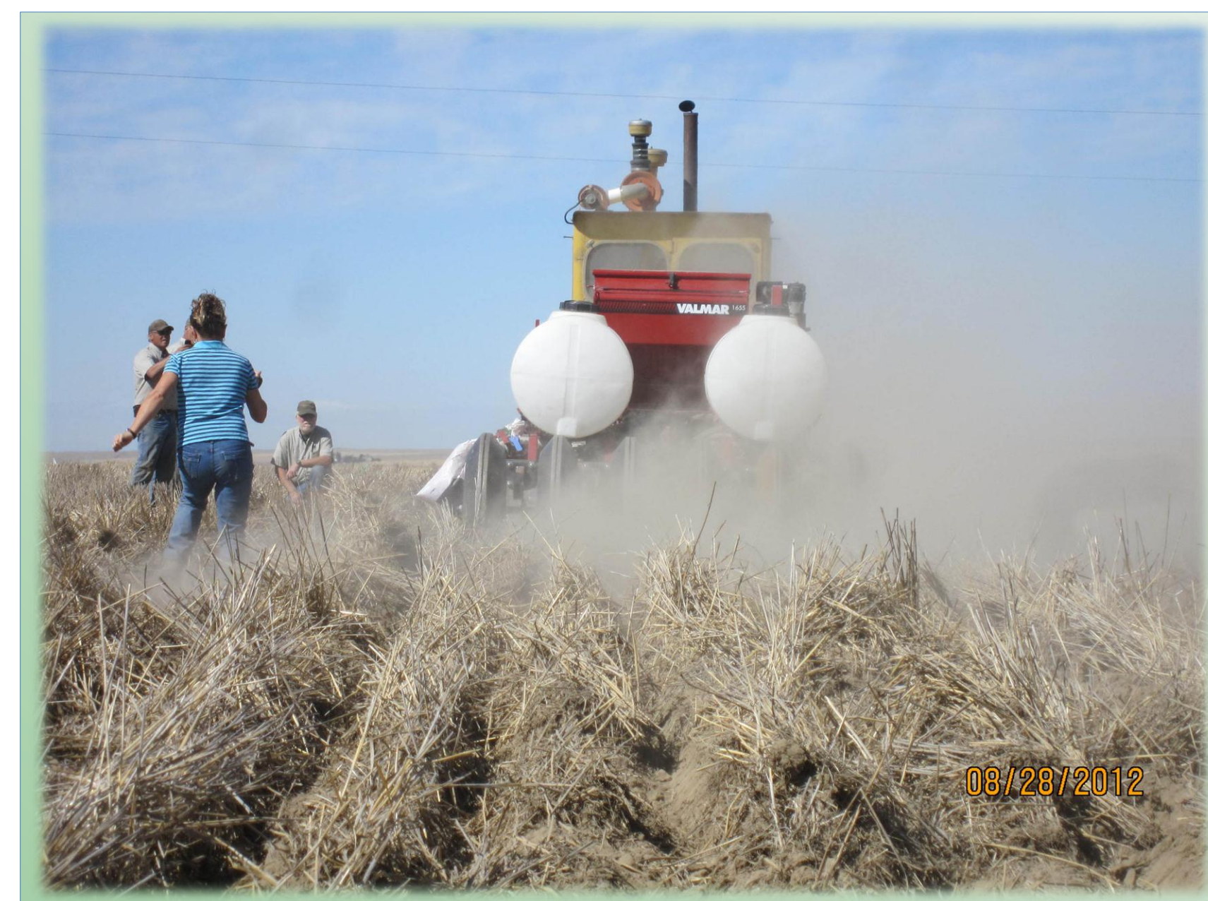
Fig. 1. Concurrent with the row spacing experiment, new deep-furrow drill prototypes are being developed that can pass through heavy residue with excellent seed placement in tilled summer fallow. This high-frame-clearance prototype has 17-inch row spacing with shovel-type openers on two ranks and had no plugging problems in three years of testing.
