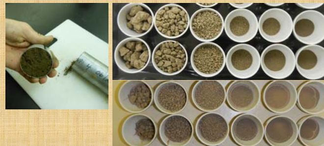
Figure 2. Particle size distribution in intact, coarsely-aggregated, and pulverized sample forms (crucible inside diameter 38 mm).
