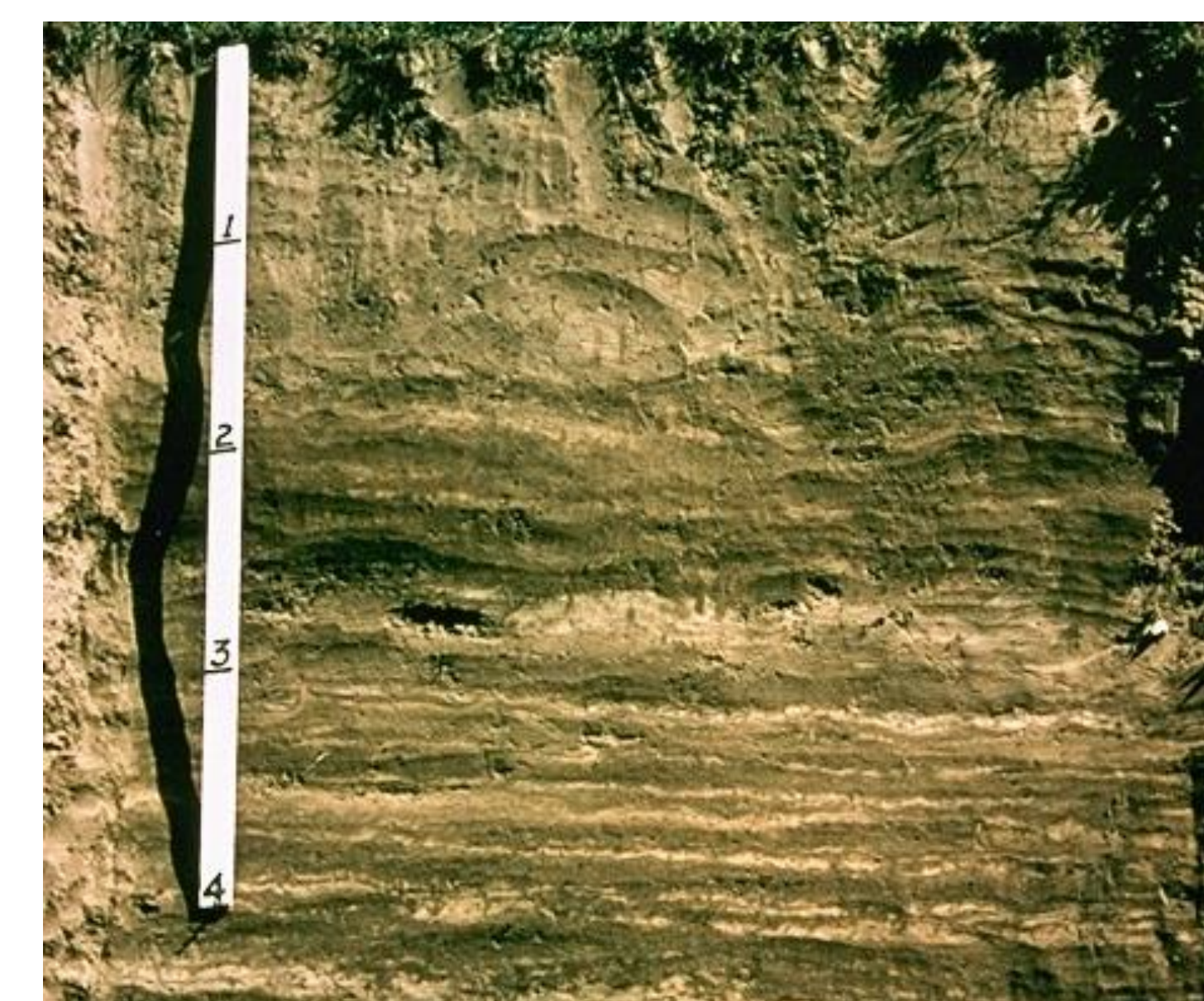
Figure 4. A Fluvent, showing the characteristic layering of floodplain deposits. Scale is in feet. Photo from the SSSA Marbut Memorial slide collection.
