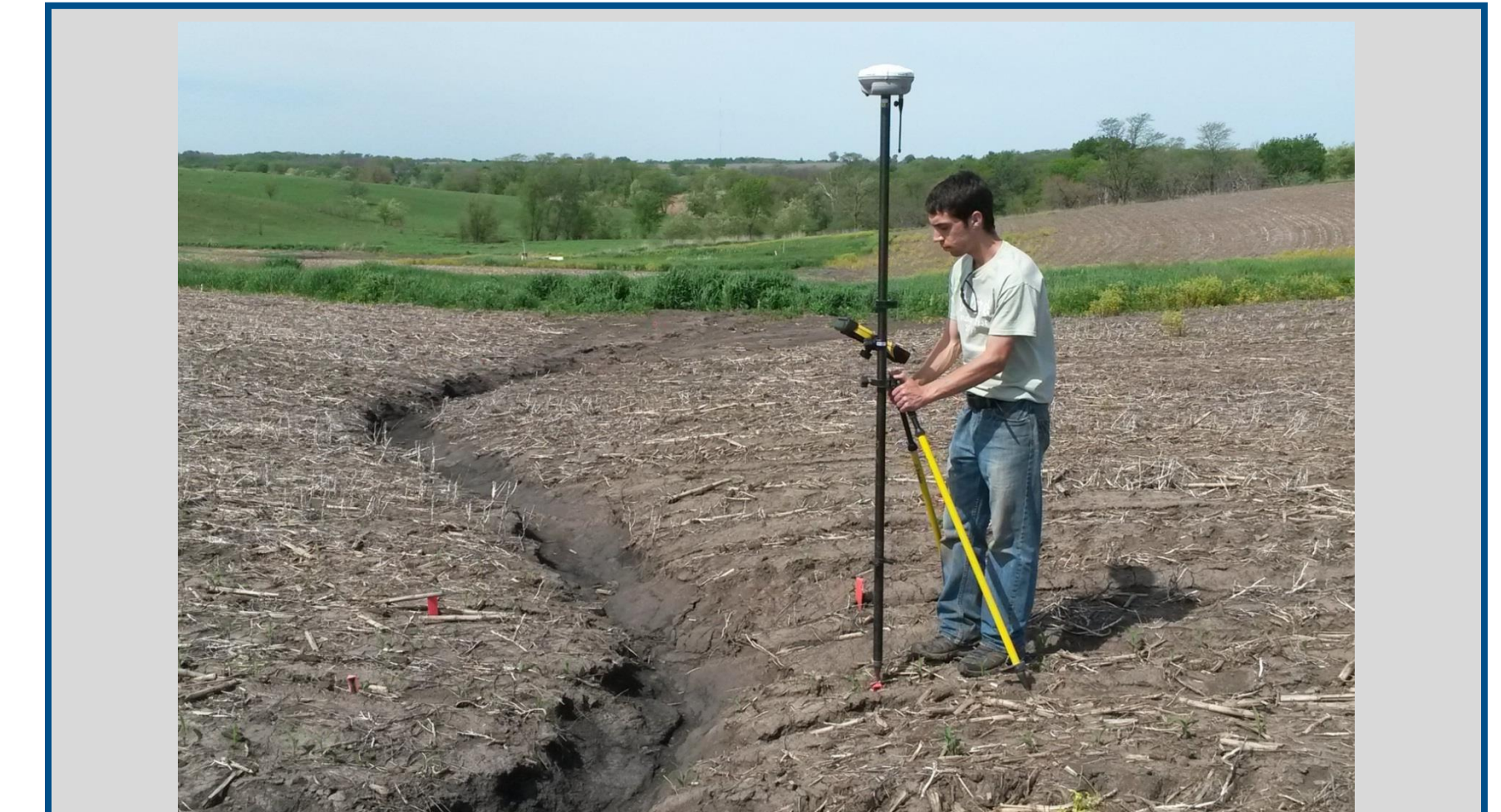
Fig 7. Surveyed control points were used to geo-reference photogrammetric point clouds.
