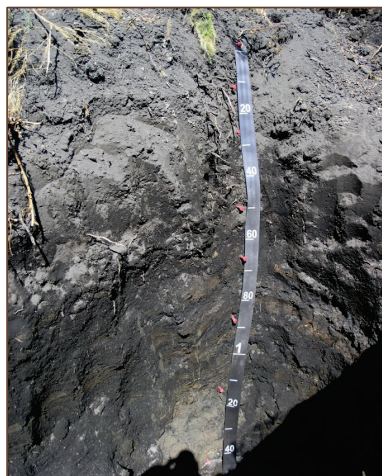
Figure 2. Pedon 13N3985. Sampled as Rindge. Correlated as fine, mixed, thermic, Histic Endoaqualf.
