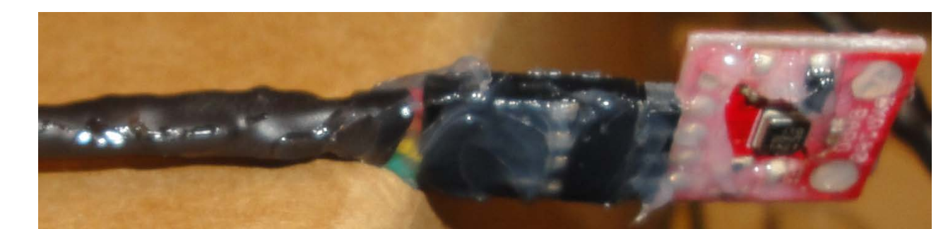
BMP 180 sensor coated with silicon
