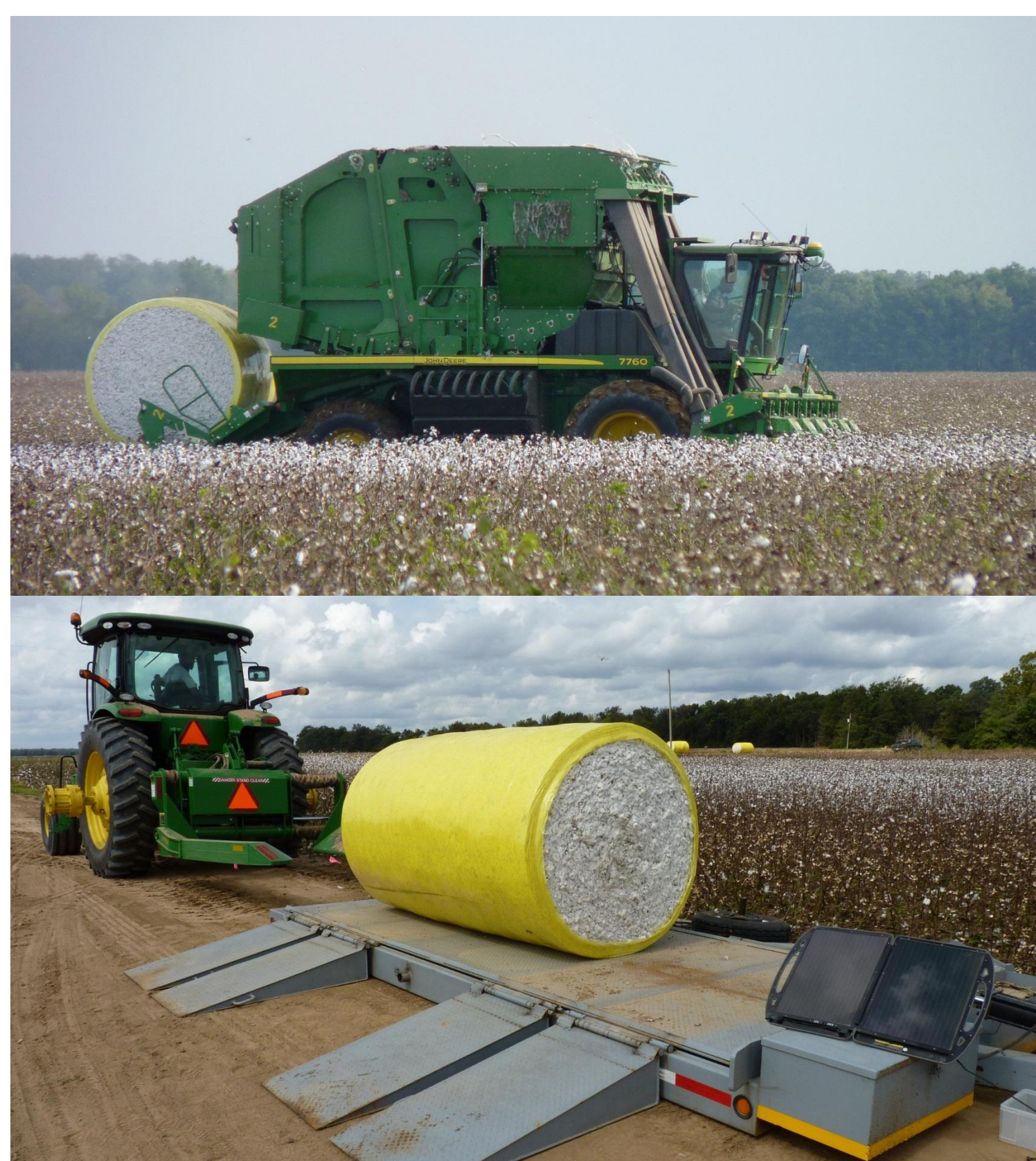
Fig. 1. Six-row cotton picker with round module builder. Trailer scale used to weigh round modules.
