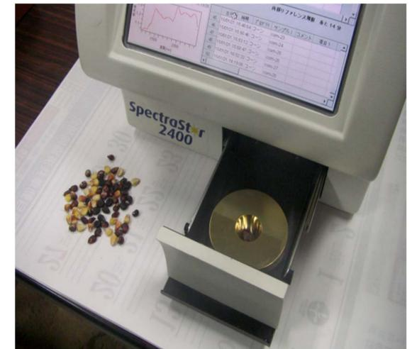
Figure1. NIR spectrophotometer equipped with a single kernel adapter (dent  $\phi$ =2.7cm).
