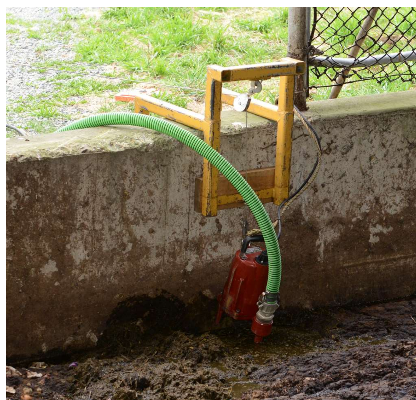
Submersible pump showing grinder knife, and in action lowered into manure storage via pulley and metal frame
