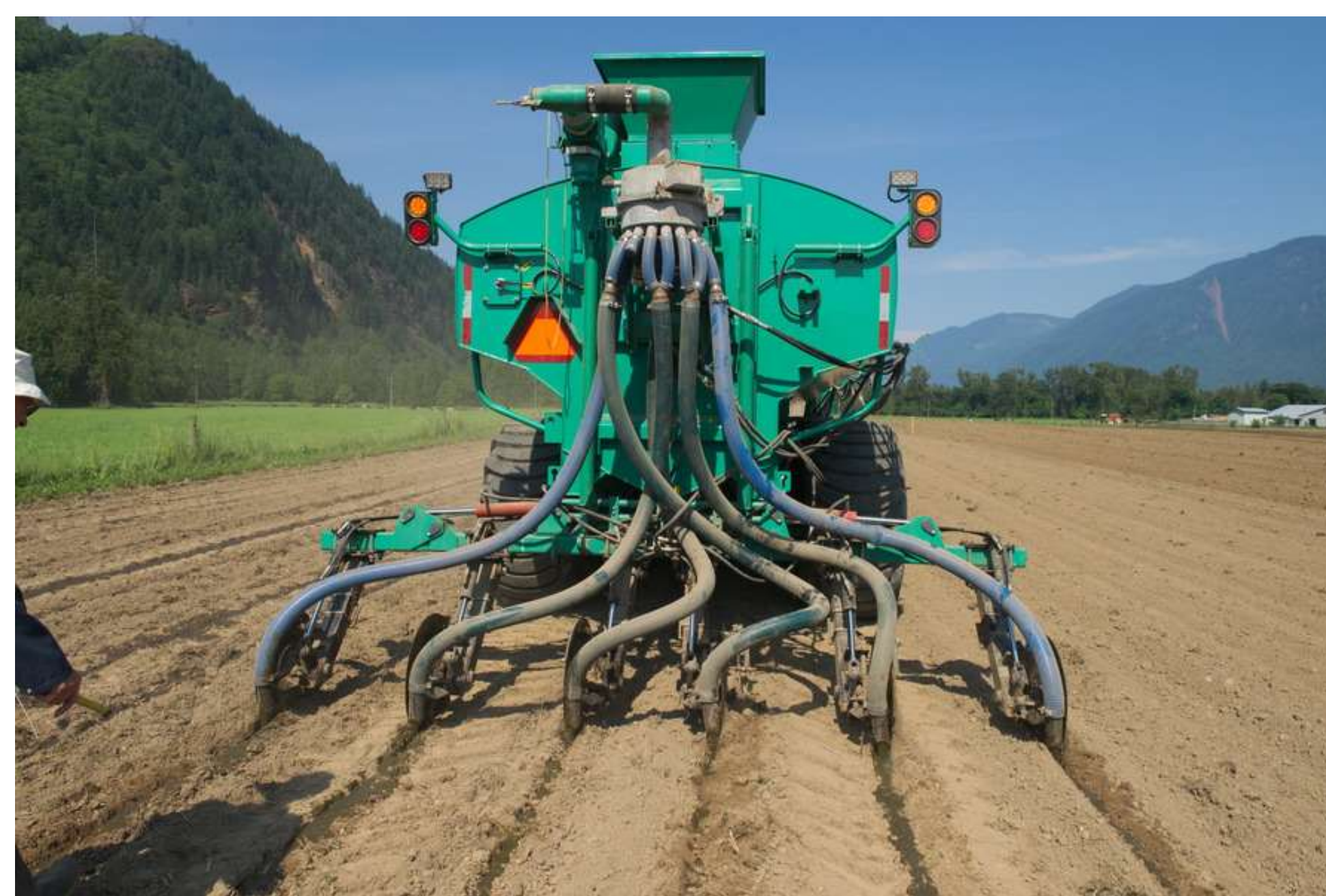
Thicker slurry precision injected several days prior to corn planting. Corn is planted over injection furrows. Higher concentration P from manure eliminates need for starter P fertilizer.
