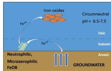
Figure 1. The biological process by which FeOB oxidize ferrous iron (Fe<sup>2+</sup>) into ferric iron (Fe<sup>3+</sup>) forming iron oxides.
