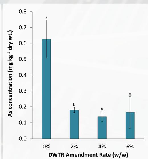
Figure 4. Mean As concentration of *B. pekinensis* aboveground tissues grown in sandy soil with band-applied P fertilizer as a function of alum-based DWTR amendment rate (0-6% w/w)
