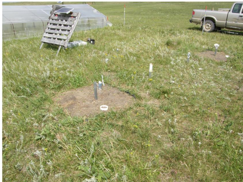
Figure 1. Field plot in the heavy grazing site, showing two trenched sub-plots (with neutron probe tubes and respiration collars) and two untrenched ones in between under natural (control) conditions, as well as a partial view of the  $3 \times 6 \text{ m}^2$  rain-out-shelter.
