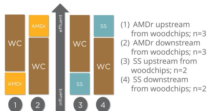
Fig. 2: Flow configurations of N (woodchips-WC) & P (acid mine drainage-AMDr; steel slag-SS) removal pairings.
