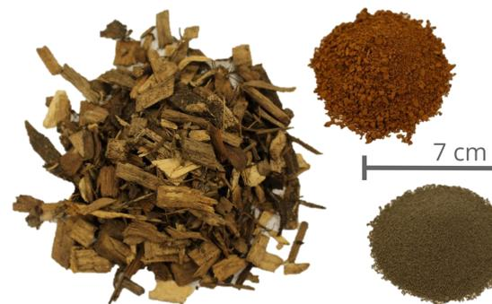
Fig. 4: (from left, same scale) N removing woodchips and P removing AMDr and SS.
