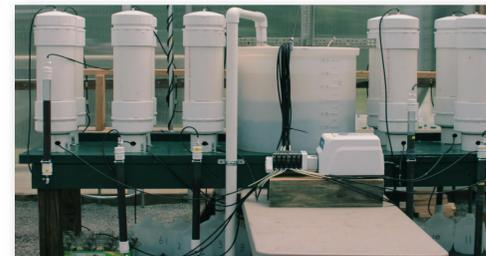
Fig. 3: Woodchip columns (white PVC) paired with P-sorbing filters (clear PVC).
