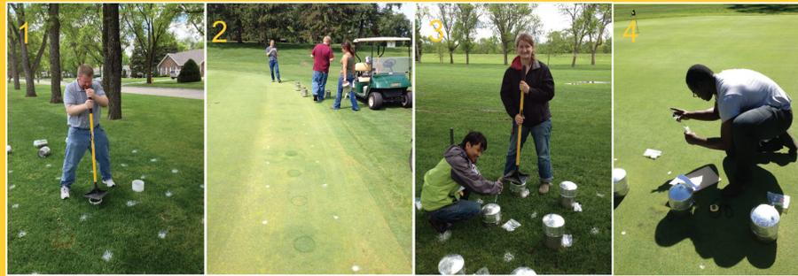
Photo 1. Anchors for each plot were tamped into the soil at the beginning of the study to provide a base for the gas chambers. Photo 2. Plot layout of the putting green with anchors installed into the turf root zone. Photo 3. Prior to sampling for greenhouse gases, the gas chambers were tamped onto the anchors to create a good seal. Photo 4. Gas samples were taken at 0, 20, and 40 minutes post closure of the gas chamber and anchor.
