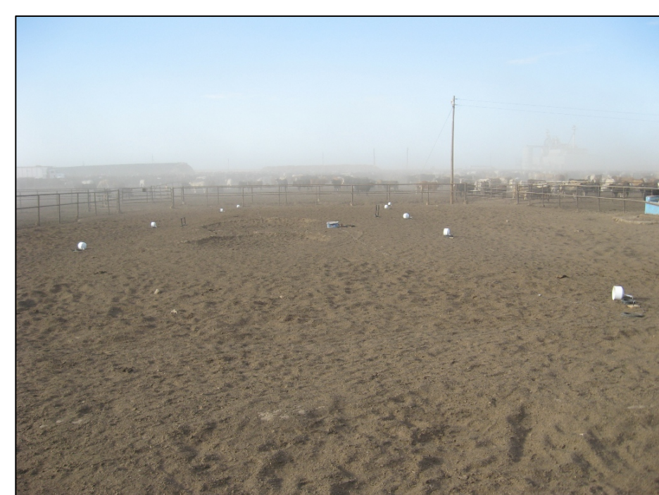
Figure 4. Two rows of five NFT-NSS chambers installed in a pen.
