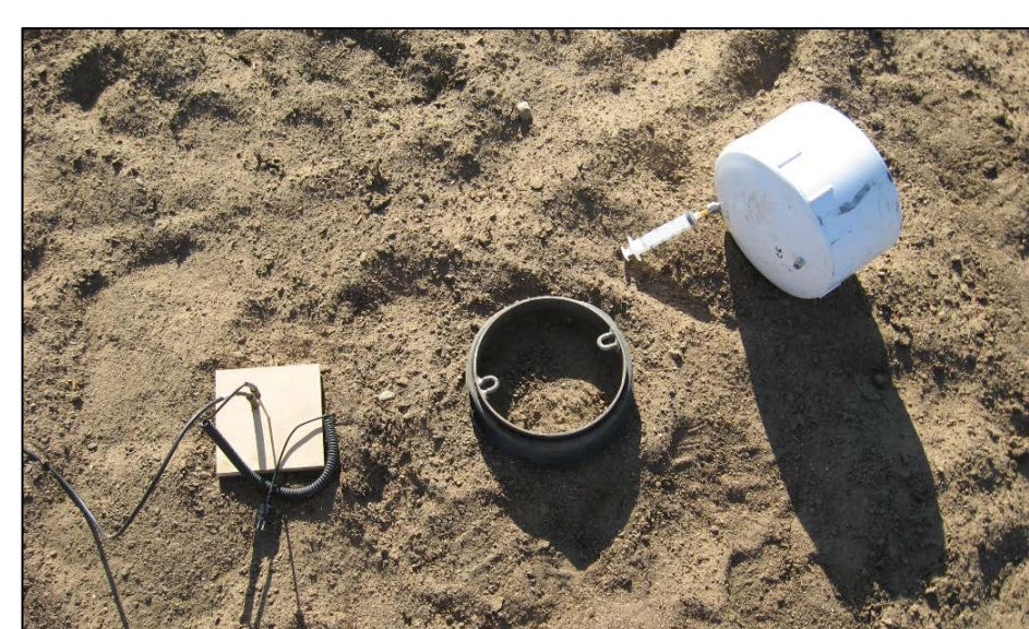
Figure 1. View of NFT-NSS chamber and base with temperature sensors installed adjacent to the base.
