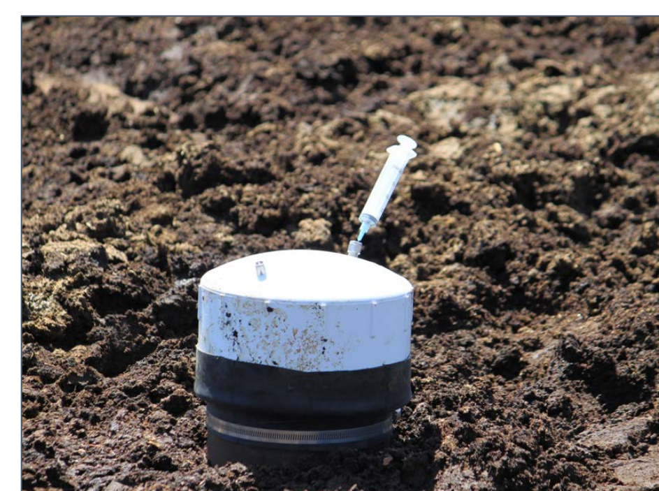
Figure 3. NFT-NSS chamber with top installed and sealing skirt rolled up.
