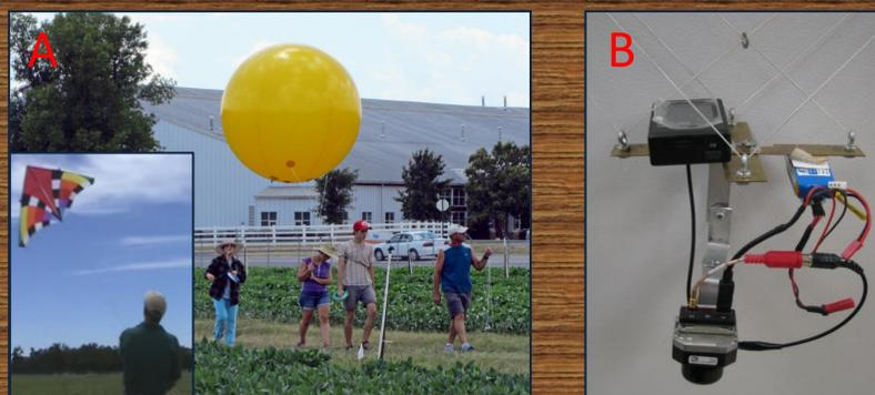
Figure 1. (A) Balloon or kite platform for aerial image and (B) picavet for the thermal infrared camera. Infrared camera with picavet was lifted 50 to 75 m above experiments using either a large tethered balloon or a kite.
