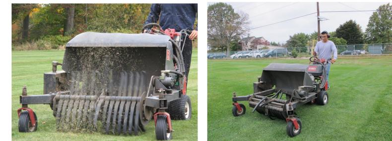
The abrasive wear applied by Rutgers Wear Simulator (RWS) causes crushing and tearing on turf plot
