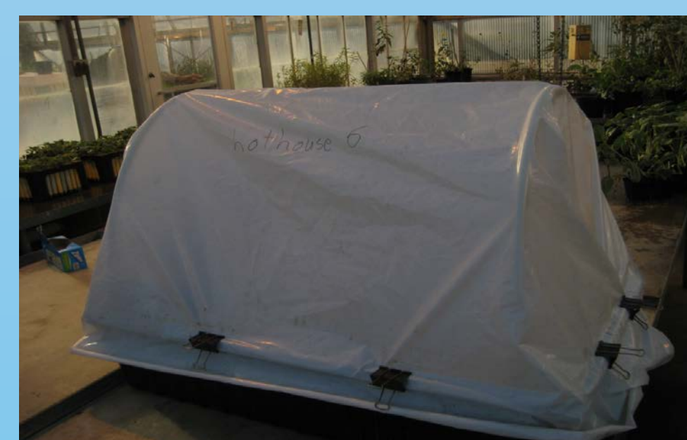
A finished humidity tent with the plastic sealed at the sides and ends with 2 inch paper clamps.
