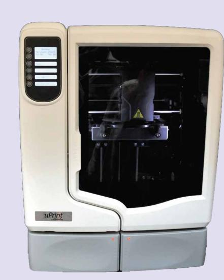
The 3-D printer uses a spool of plastic which is fed to a nozzle where it is melted and laid down one 250-µm layer at a time to "print" the specimen from the bottom up.
