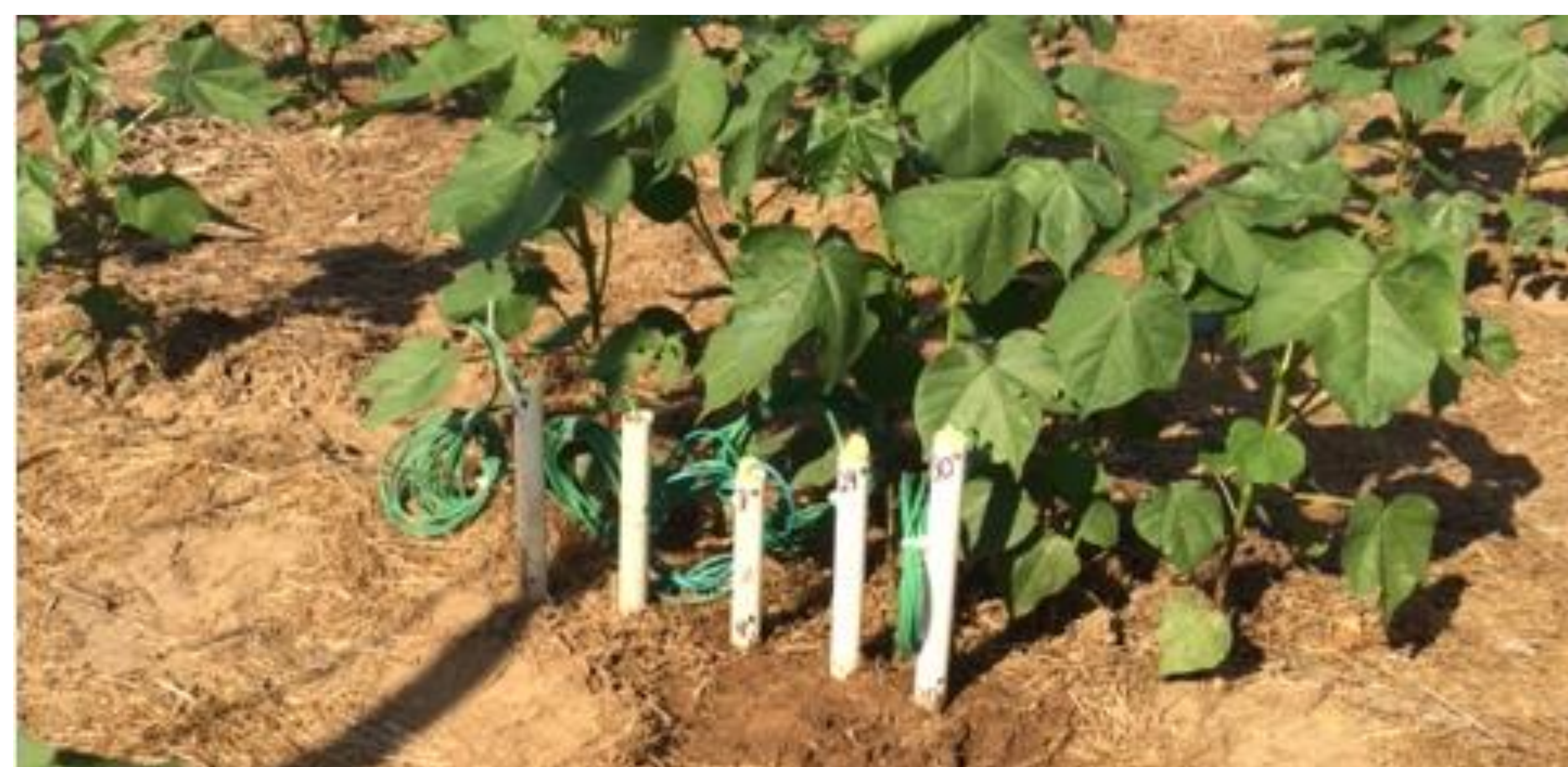
Figure 1. 5 Watermark soil moisture sensors installed at depths of 15, 31, 46, 61, and 76 cm to validate rooting depth.
