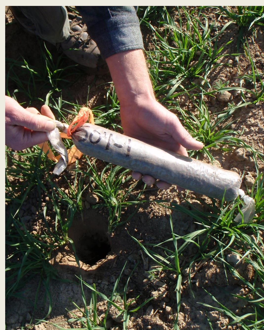
Fig. 1. To monitor N mineralization rates after field applications of dairy cattle manure, manured soils were placed in plastic bags and buried in the field. Throughout the growing season the bags were removed and analyzed for nitrate and ammonium. The buried bags function as in-situ incubation containers, protecting soils from plant N uptake and leaching of N.
