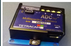
Tetracam ADC-Snap sensors with RGB and CIR cameras were flown over field after every week to collect UAV images.
