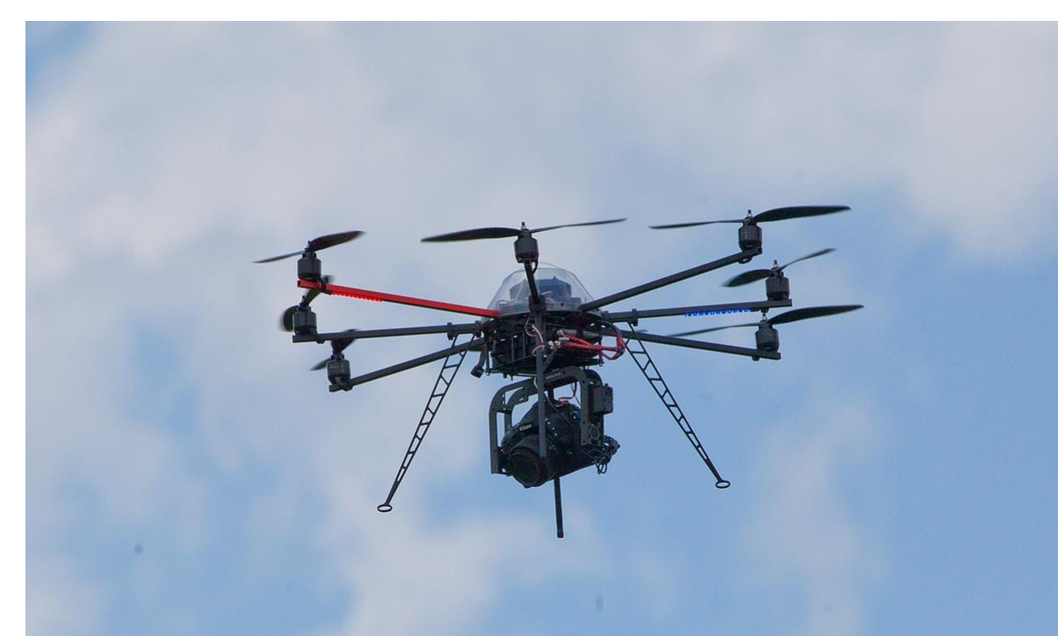
Figure 1: The octacopter platform used to capture our aerial multispectral images.
