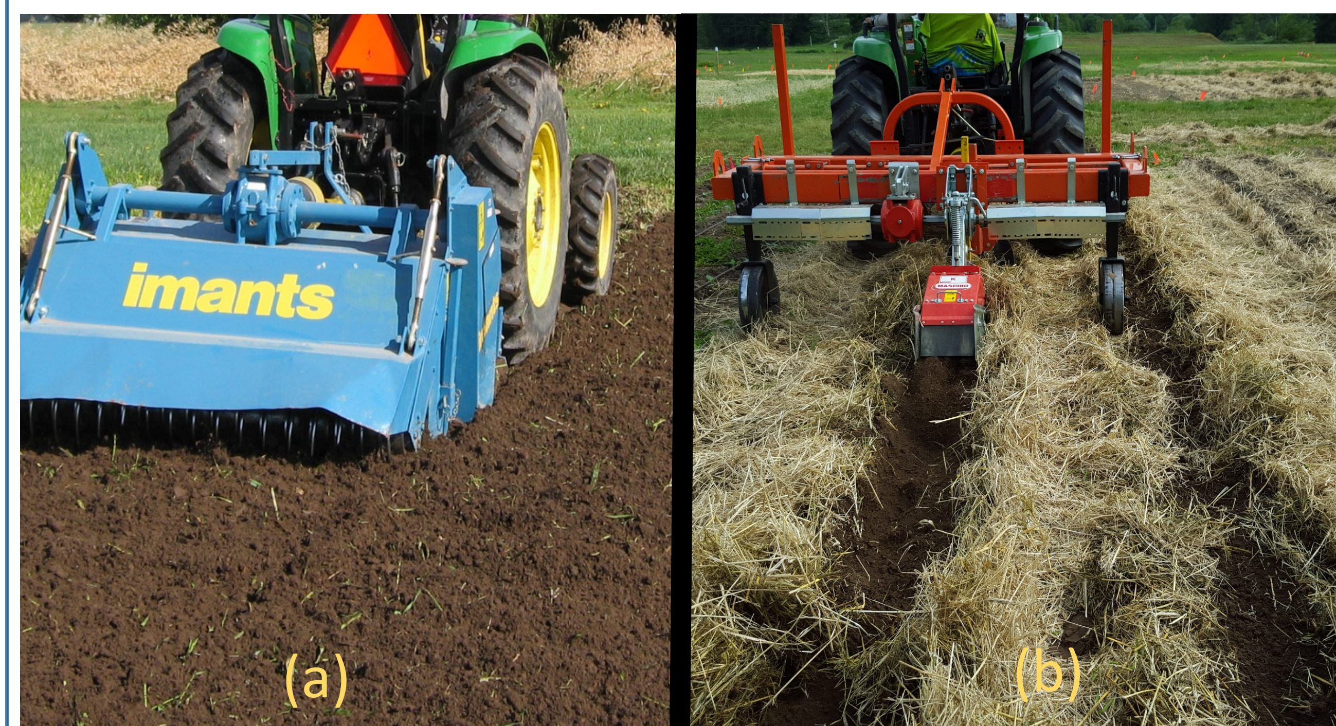
Figure 1: Imants rotary spader used in full till treatment (a) and modified Maschio powered strip tiller and strip tilled rye residue (b) prior to mechanical transplanting.
