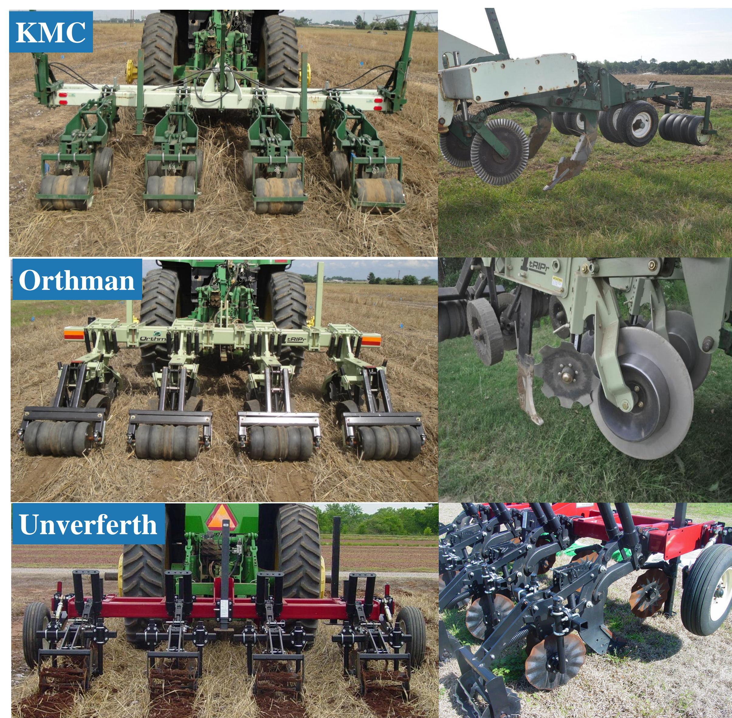
Fig. 1. Strip tillage implements, corresponding shanks, and attachments used in the cover crop, row pattern study for peanut during the 2012-2014 growing seasons at Headland, AL and Tifton, GA. Tillage depths were ~33 cm for the implements.
